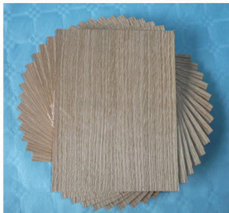
Figure 7. A twisted wood model made from oak sheets. Every consecutive sheet is rotated for a fixed angle regarding to precedent sheet. (Figure appears in color online.)
